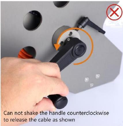
Can not shake the handle counterclockwise to release the cable as shown
